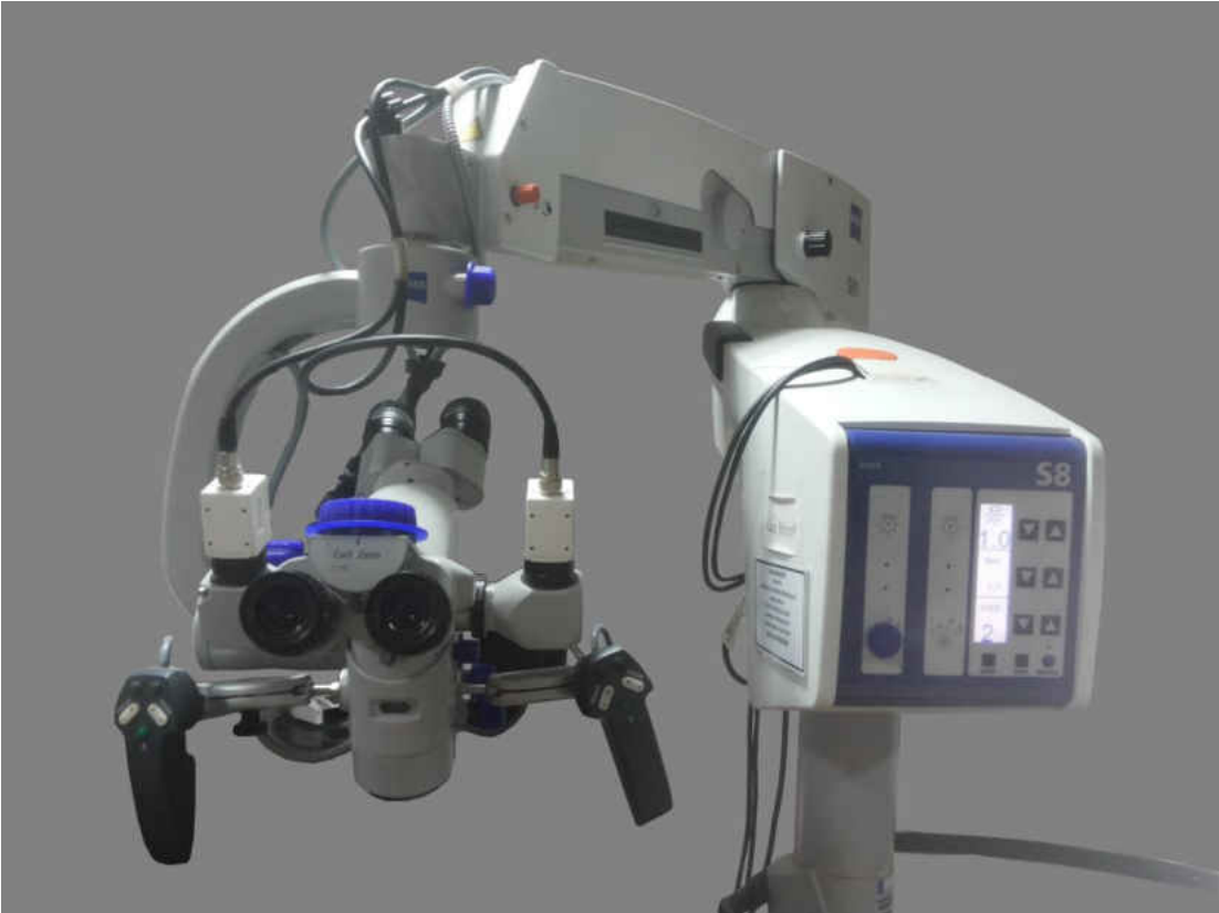
Figure 2.1-1 - Operating Microscope with a beam splitter, adapter and cameras for the acquisition purpose
