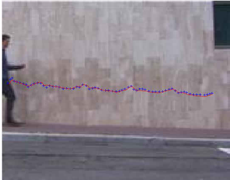
Figure 2.2.9-1 - Tracks: Centroid locations measured by the Algorithm are shown in blue and ground truth shown in red
