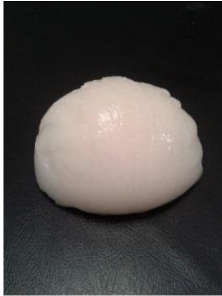
Figure 15. Solid phantom simulating the human breast tissue
