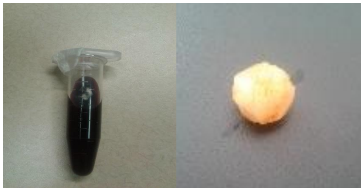
Figure 16. Ferrofluid containing the nanoparticles and tumor phantom
