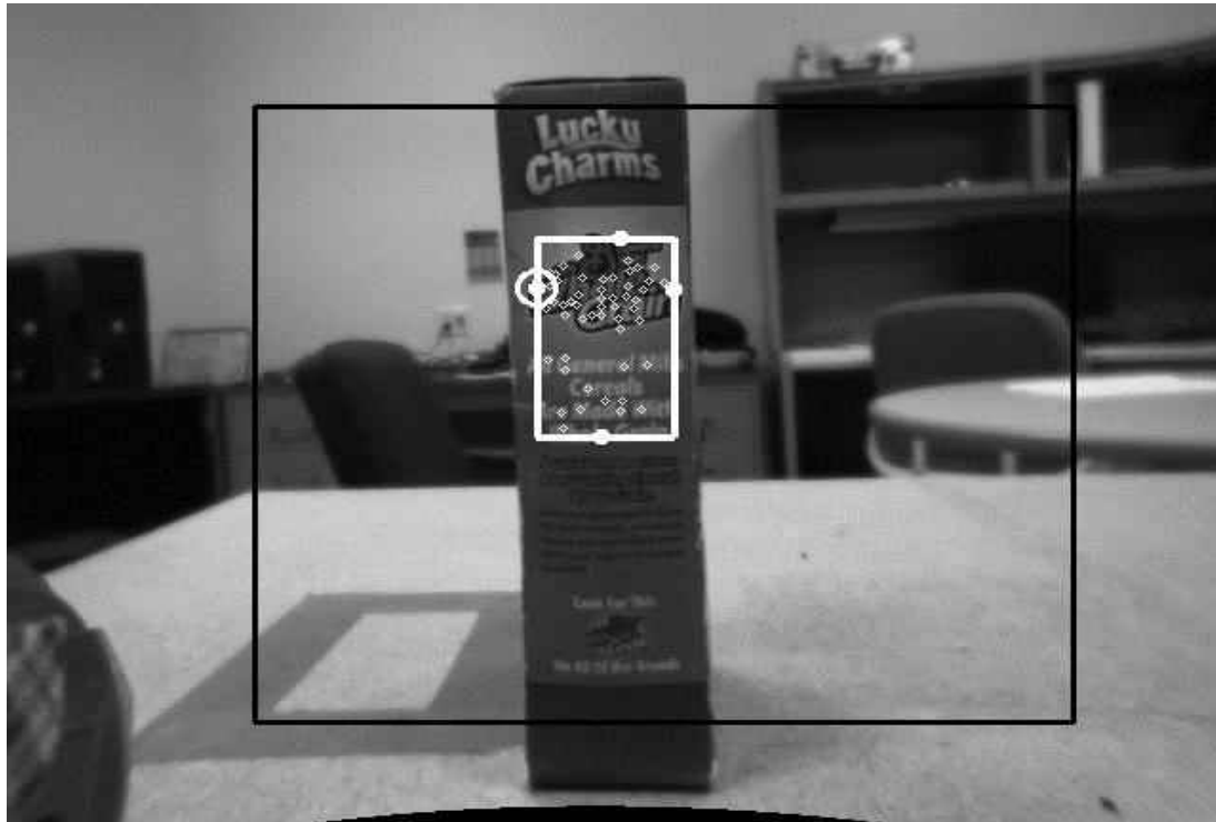
Figure 3-1: Initialization step for Fine Motion artificial ROI (black) around the object
