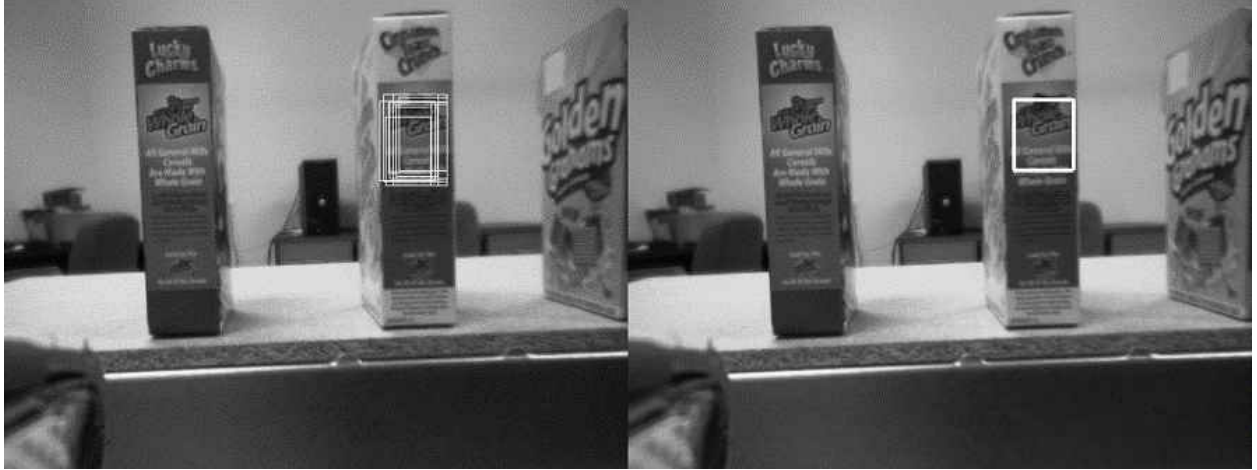
Figure 5-1: Particles ROIs (left) and output ROI (right) in frame 42 of a cereal-box video sequence recorded in the UCF Assistive Robotics Laboratory.
