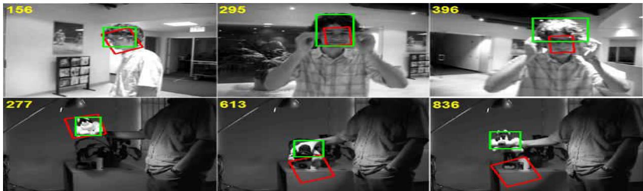
Figure 5-8: Sample comparison of results from IL tracker (red) to proposed method (green) on Dudek sequence.
