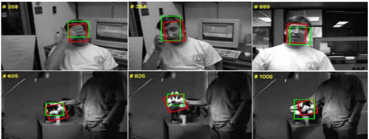
Figure 5-10: Sample comparison of results from TOT method (red) to proposed method (green) on the Dudek (top) and Sylvester (bottom) sequences.
