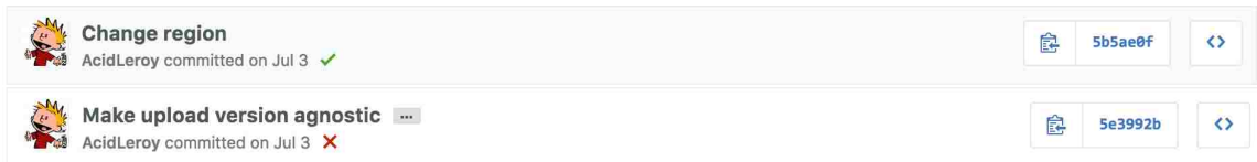
Figure 3.8: An example of two commits that were pushed to our repository. The top figure shows how the build is marked as passing with a green check mark, and the bottom shows the build failing with a red x.
