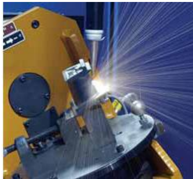
Figure 1.13 A LASER drilling holes into a blade surface (Courtesy Primal/Laserdyne)
