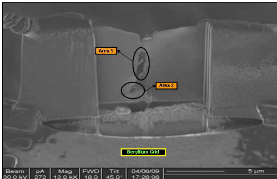
Figure 41. FIB G.B. Cut - In-Situ sample extraction containing voids
