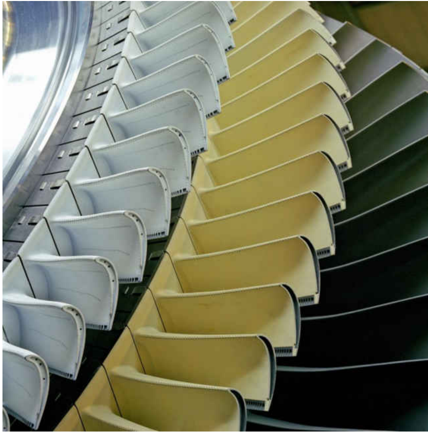
Figure 1.4 - Turbine layers one to three of a 292+ MW Siemens SGT5-4000F Gas turbine. Thermal barrier coatings (TBC) and careful material design and selection allows operation at combustion exit temperatures of 1400°C for this turbine. [10]
