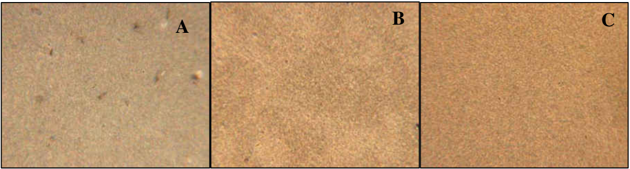
Figure 5.2: Optical images (@ 50x) for CIGSe samples with A) No NaF, B) 40 Å NaF and C) 80 Å NaF
