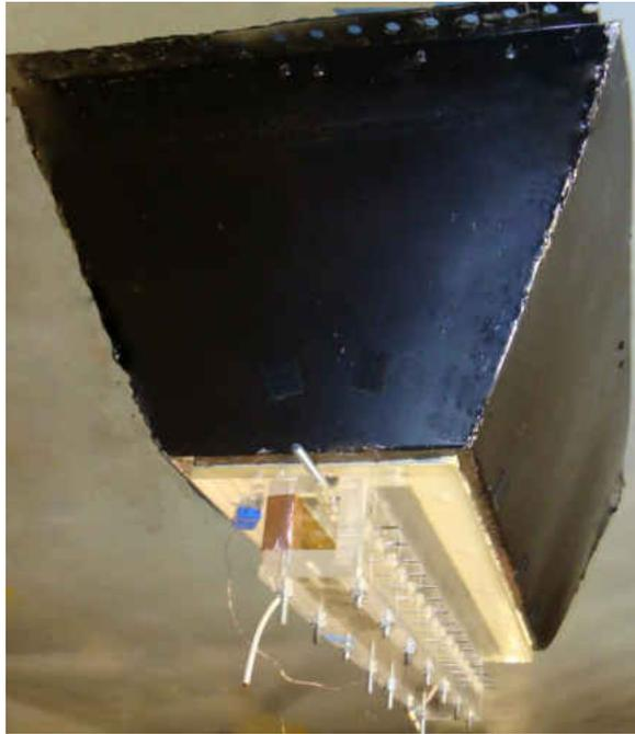
**Figure 3-10: Assembled Suction Test Section**
