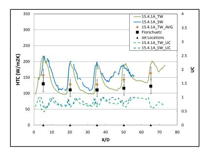
Figure 7-44: Span-averaged uniformity and heat transfer distribution (15.4.1A)
