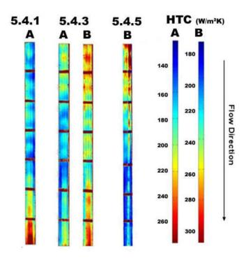
Figure 7-3: Impingement Plate HTC
