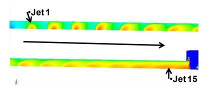
Figure 5-17: Target wall heat transfer coefficient contours
