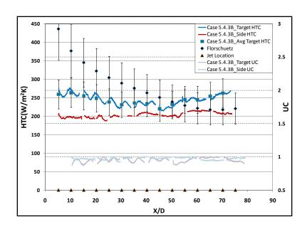
Figure 7-39: Span-Averaged Uniformity and Heat Transfer Distribution (Case 5.4.3B)
