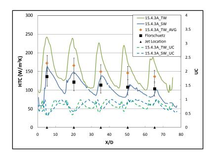
Figure 7-45: Span-averaged uniformity and heat transfer distribution (15.4.3A)
