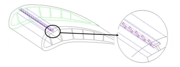
Figure 3-1: Peripheral Cooling Details
