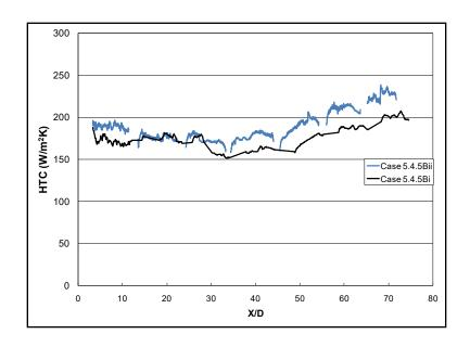
Figure 7-25: Heating Variation Effects: Case 5.4.5 Side Wall
