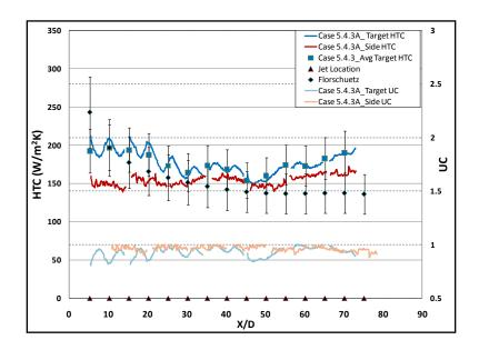
Figure 7-38: Span-Averaged Uniformity and Heat Transfer Distribution (Case 5.4.3A)
