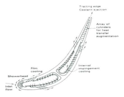
Figure 1-2: Turbine Blade Cooling Techniques (Taylor, 1980)
