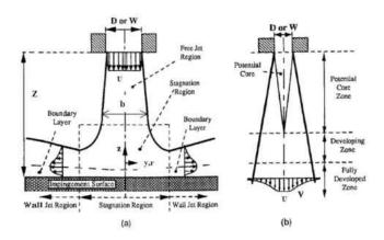
Figure 2-1: Hydrodynamics of Impinging Flow (Viskanta, 1993)
