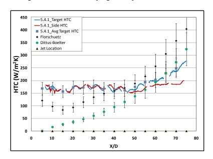
Figure 7-26: Span-averaged literature comparison (5.4.1A)
