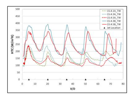
Figure 7-9: Span-averaged Target Wall Heat Transfer Distribution (X/D=15)
