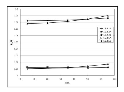
Figure 6-6: Pressure Ratio Distribution (X/D=15)
