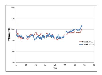
Figure 7-21: Heating Variation Effects: Case 5.4.1 Side Wall
