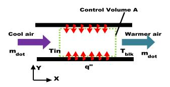
Figure 7-12: Standard Steady State Energy Balance
