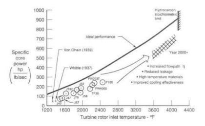
Figure 1-3: Turbine Inlet Temperature versus Power (Sautner et al., 1992)
