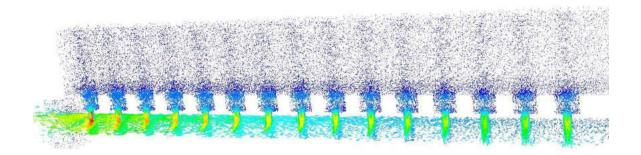
Figure 5-11: Impingement Channel Velocity Vectors
