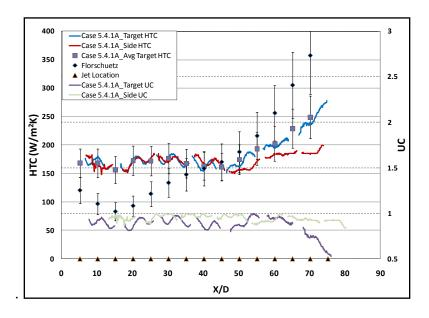
Figure 7-37: Span-Averaged Uniformity and Heat Transfer Distribution (Case 5.4.1A)
