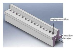
Figure 3-2: Test Section Geometry
