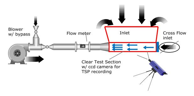
Figure 3-9: Suction Driven Flow Loop
