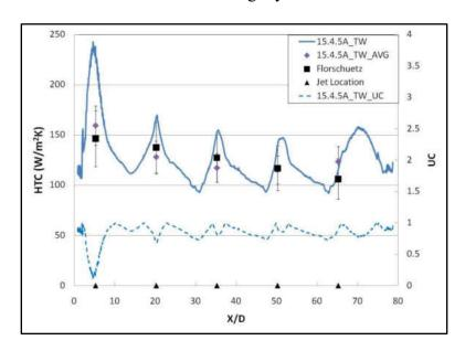
Figure 7-47: Span-averaged uniformity and heat transfer coefficient (15.4.5A)
