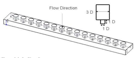
Figure 3-3: Jet Plate Geometry
