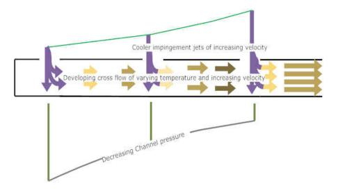
Figure 1-6: Impingement Channel Flow Scenario
