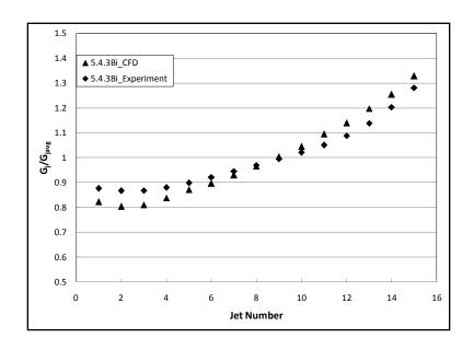
Figure 5-5: Normalized Mass Flux Comparison
