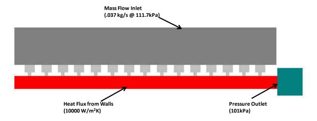
Figure 5-3: CFD Boundary Conditions
