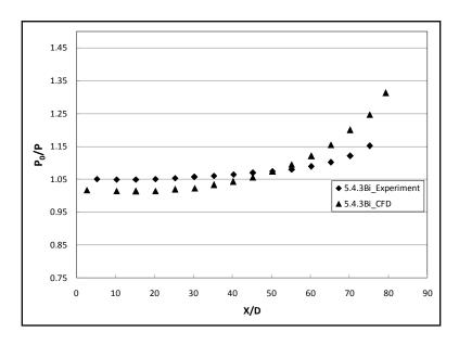
Figure 5-4: CFD Pressure Ratio Comparison
