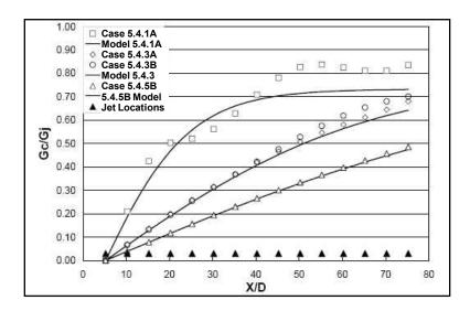
Figure 6-4: Normalized Cross flow Mass Flux Distribution
