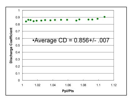
Figure 6-1: Jet Plate Discharge Coefficient
