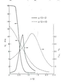
Figure 2-3: Z/D effect on turbulence and velocity (adapted from Hoogendoorn, 1977)
