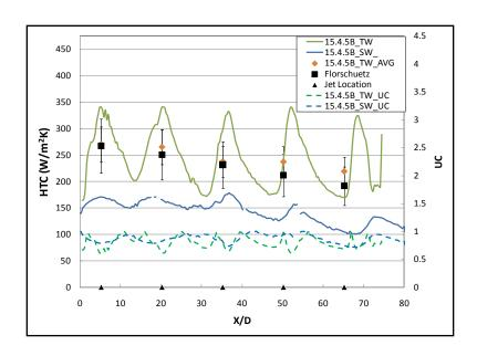
Figure 7-48: Span-averaged uniformity and heat transfer coefficient (15.4.5B)
