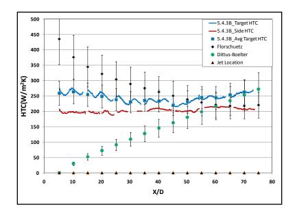
Figure 7-28: Span-averaged literature comparison (5.4.3B)
