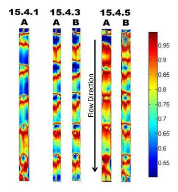
**Figure 7-42: Target Wall Uniformity Distributions (X/D=15)**
