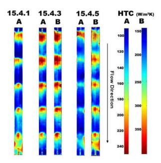
Figure 7-8: Target Wall Heat Transfer Coefficient Distributions (X/D=15)
