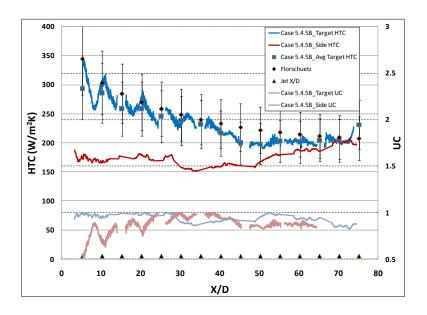
Figure 7-40: Span-Averaged Uniformity and Heat Transfer Distribution (Case 5.4.5B)
