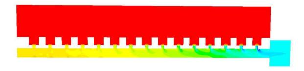
Figure 5-6: Symmetry Plane Static Pressure Distribution
