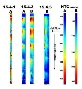
Figure 7-10: Side Wall Heat Transfer Distributions (X/D=15)
