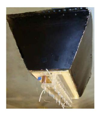
Figure 3-10: Assembled Suction Test Section
