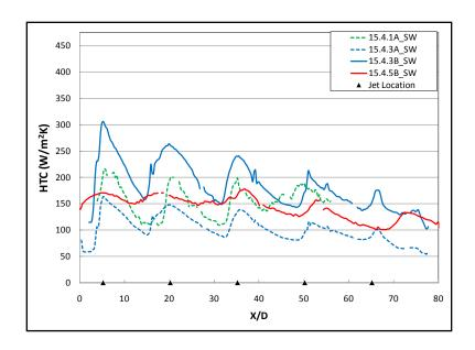
Figure 7-11: Span-averaged Heat Transfer Distribution (X/D=15)
