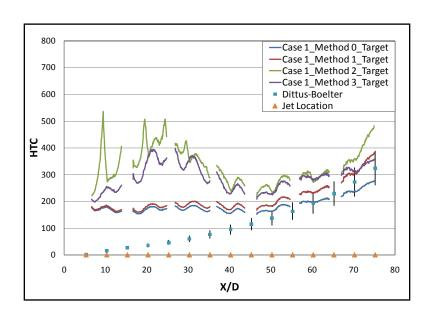
Figure 7-16: Target Wall HTC Trends- Z/D=1
