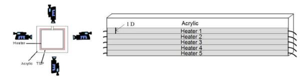
Figure 3-7: Heat Transfer Test Set-up
