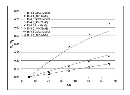
Figure 6-8: Normalized Mass Flux Distribution (X/D=15)
