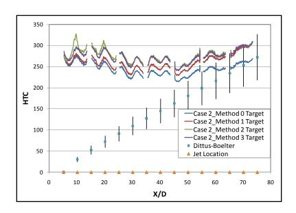
Figure 7-18: Target Wall HTC Trends-Z/D=3
