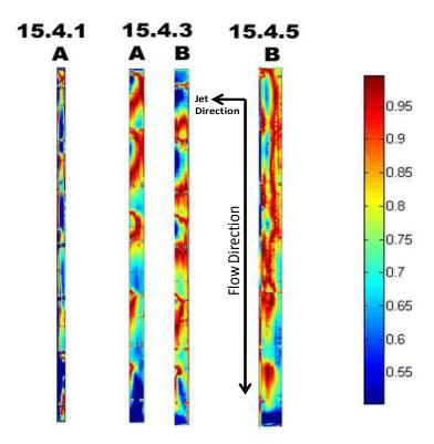
Figure 7-43: Side Wall Uniformity Distributions (X/D=15)
