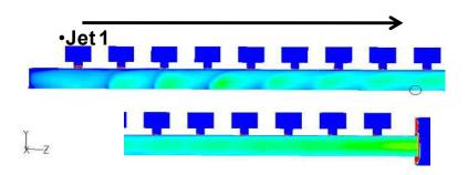
Figure 5-18: Side wall heat transfer coefficient contours
