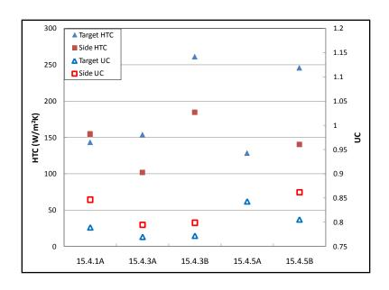
Figure 7-49: Overall uniformity and heat transfer coefficient comparison (X/D=15)
