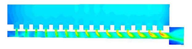
Figure 5-10: Symmetry Plane Turbulence Intensity (%)
