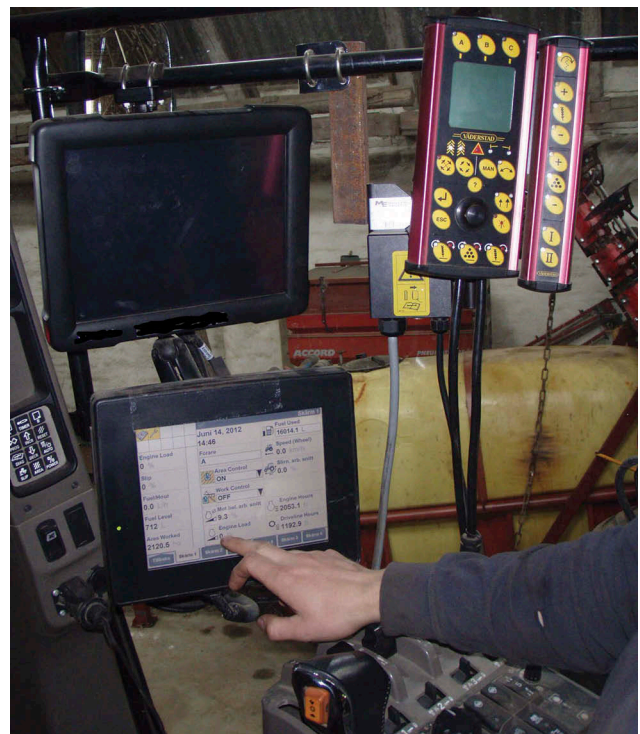
Figure 2. High-tech machines with camera surveillance, GPS monitor screen and implement control, data boxes, and joysticks.
