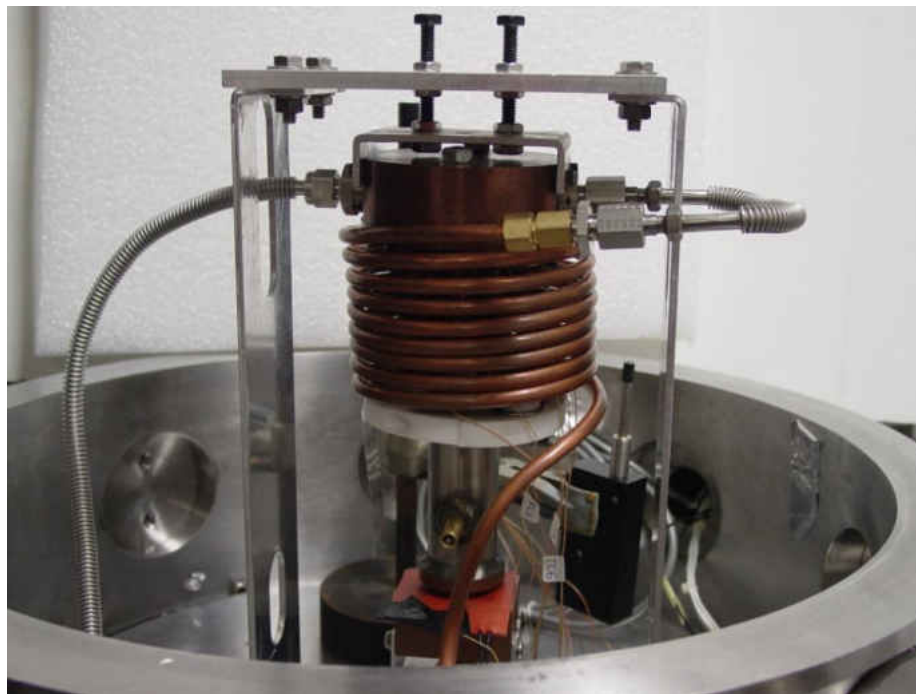
Figure 6.8: Thermal switch and single-loop cooling coils connected to liquid nitrogen lines
