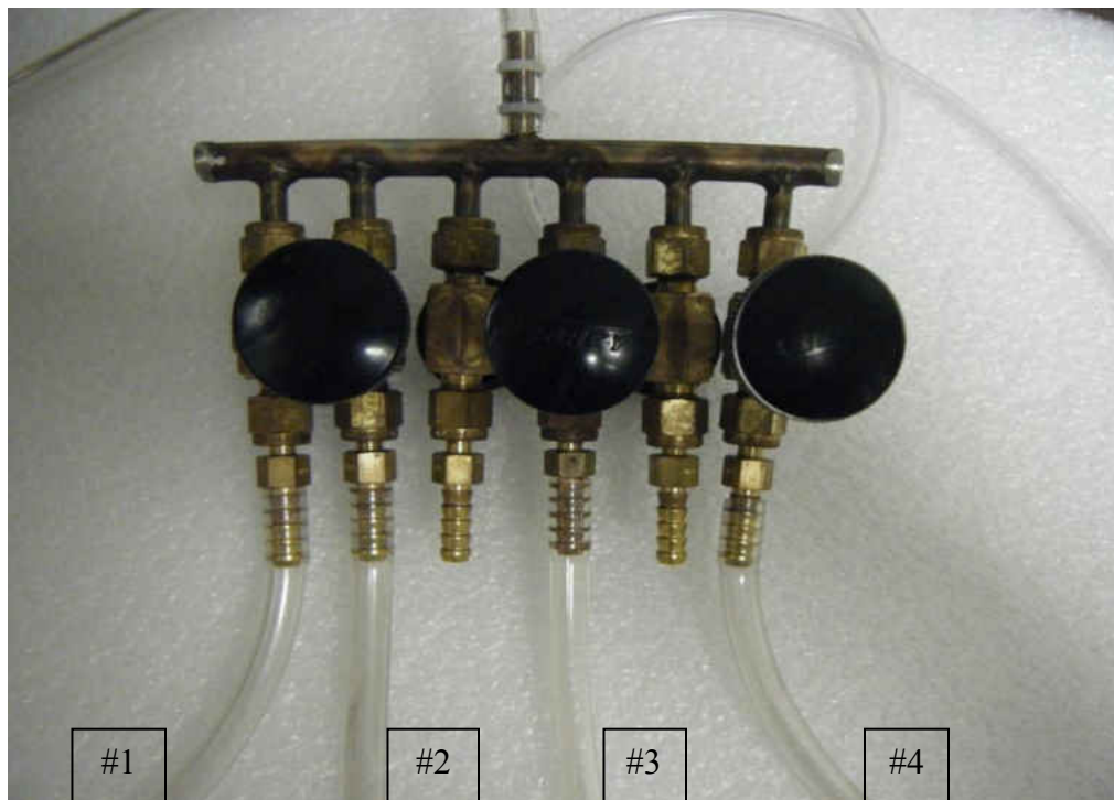
Figure 6.1: Pressure manifold for heat pipe evacuation and charging
