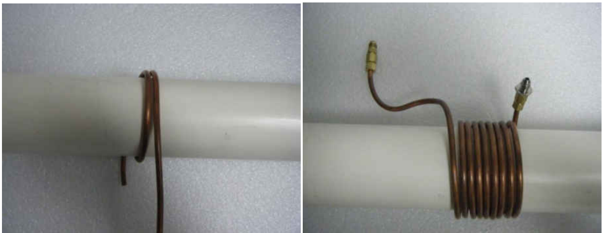
Figure 6.5: Fabrication of the single-loop cooper tube
