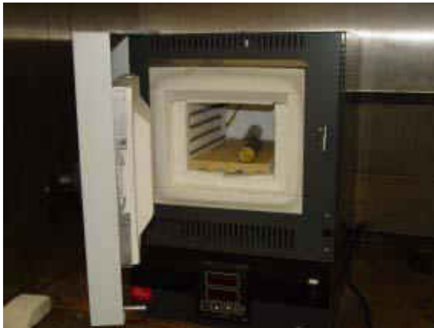
Figure 3.14: Mandrel containing coiled SMA wire in the furnace
