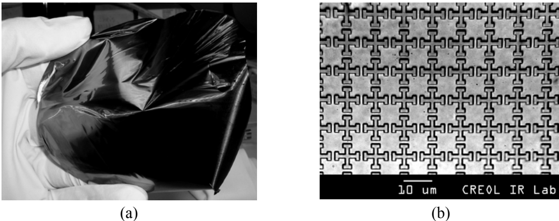
Figure 24: Completed polyimide FSS: (a) Flexible 10 cm (4 inch) wafer fully populated, (b) Elements intact on flexible substrate after polyimide backing removal.
