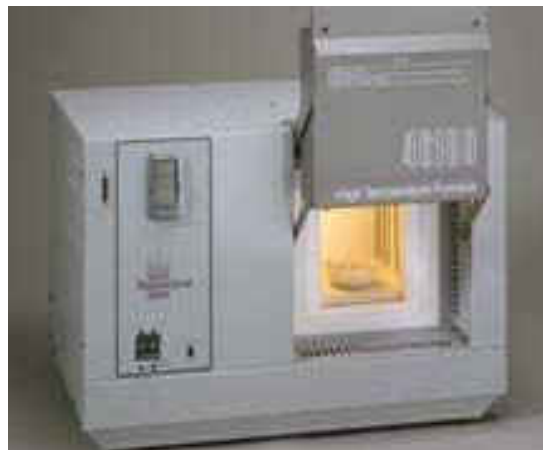
Figure 9 : High temperature furnace used for the sintering of titania structures
