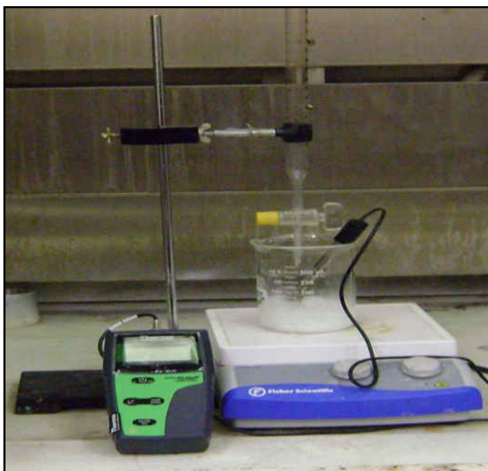
Figure 8: Setup showing the Sol-gel synthesis of nanocrystalline titania
