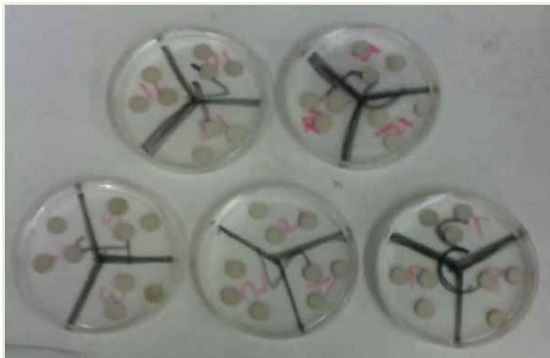
Figure 13: Setup showing titania samples placed in SBF solution
