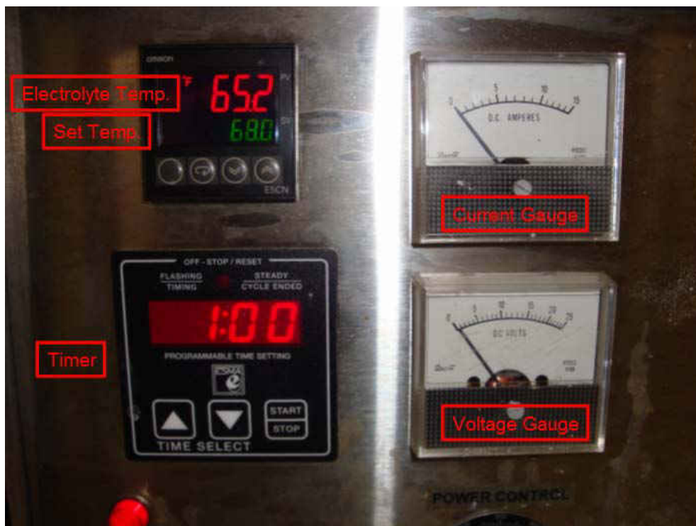
Figure 3.4: Gauges and displays on front panel of electropolisher
