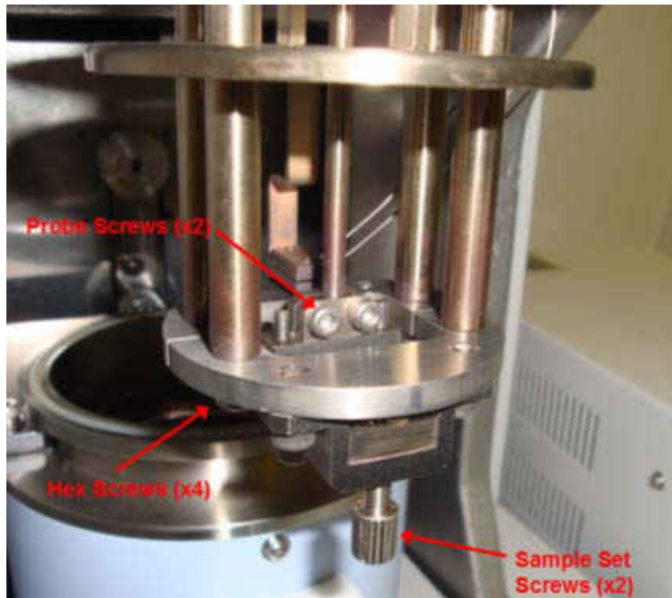
Figure 4.8: Bending fixture assembled to the DMA
