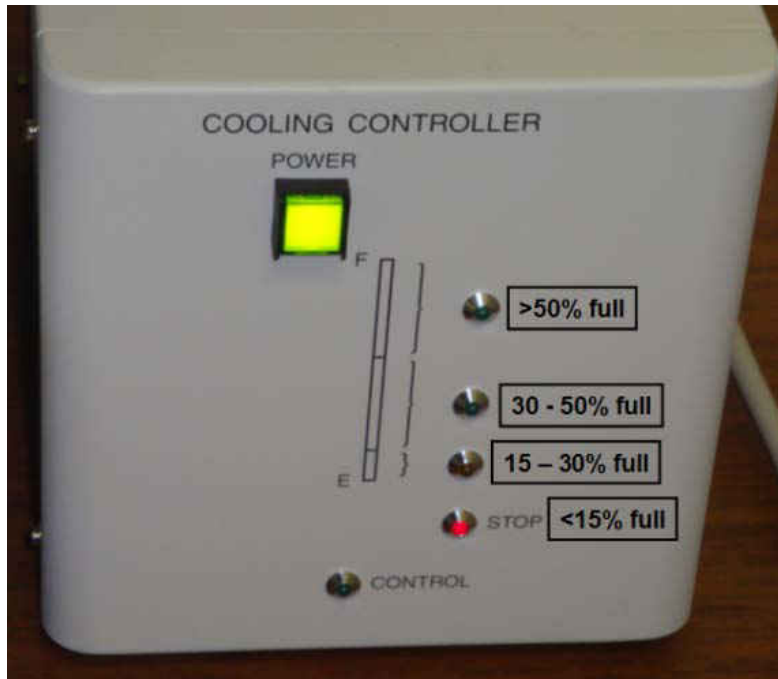
Figure 4.4: Furnace cooling controller showing fluid level indicator lights
