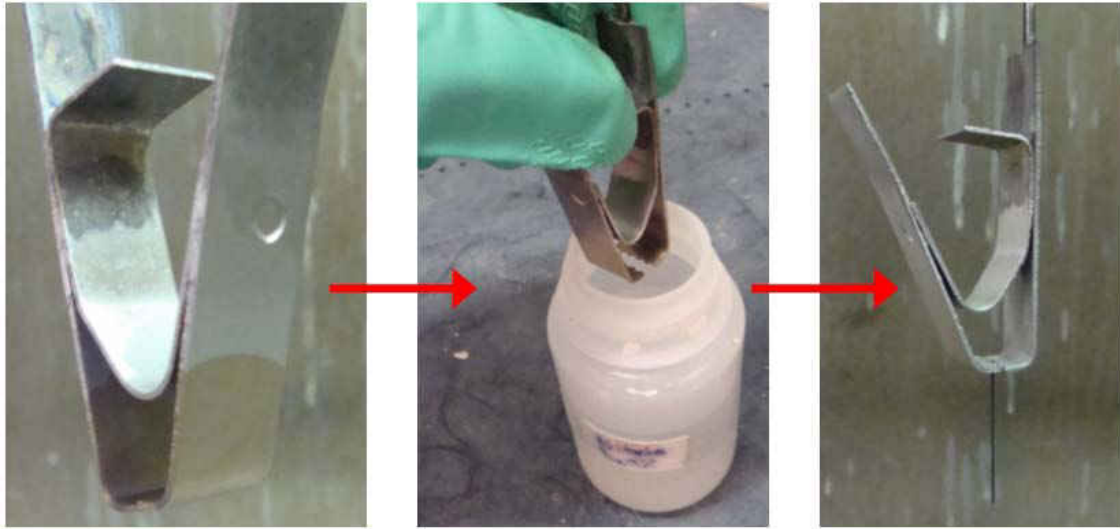
Figure 3.5: Deoxidization of titanium holding clip and placement of sample back in the clip
