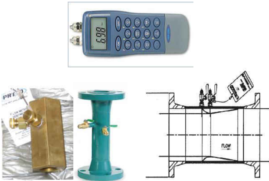
Figure 10: Venturi and pressure manometers used
