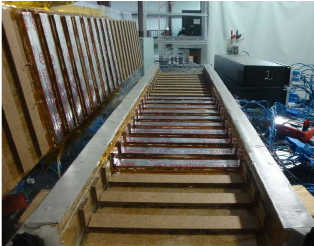
Figure 36: Case 6 repeated with taped rib surface
