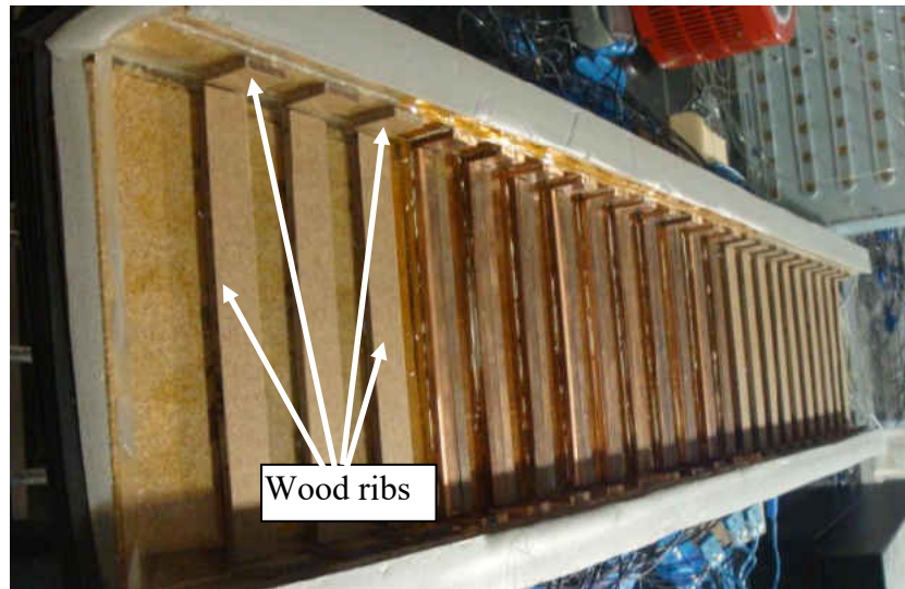
Figure 34: 1: 8 Aspect ratio channel
