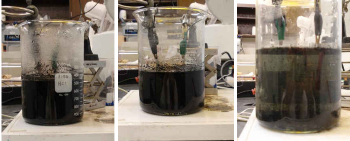
Figure 26. Precipitation of CNT in diluted copper electrolyte. (a) after sonication; (b) after 1h and (c) after 2h
