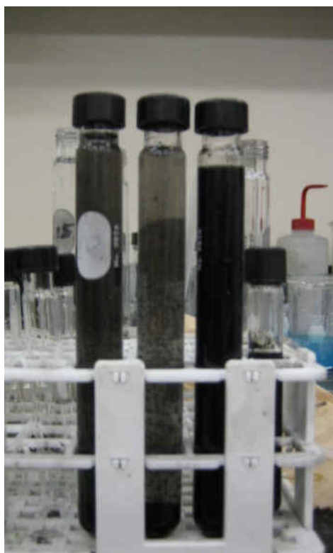
Figure 28. Dispersion of carbon nanotubes under different temperature 2 hours after ultrasonic bath
