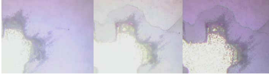
Figure 23. Beads are held at the edges of electrodes as water is removed and voltage held constant
