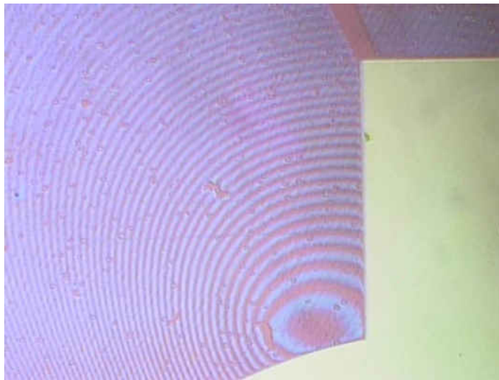
Figure 16. Irregularities caused by presence of electrodes during spin coating process
