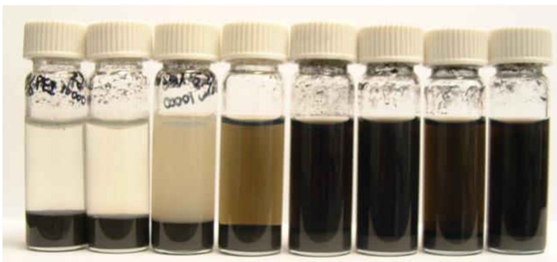
Figure 35: Sedimentation of 2 grams of W powder after ultrasonication under a power of 10 watts for 60 minutes in 5ml of PEI water solution. The PEI concentration from left to right is 2.8 %, 3 %, 3.2 %, 3.5 %, 3.9 %, 4.2 %, 4.7 % and 5 %.
