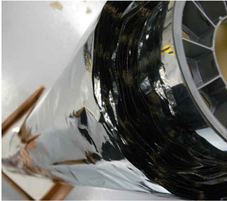
Figure 15: IMLI Cryostat-100 layup
