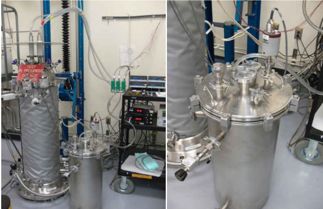
Figure 10: Cryostat-100 backpressure control system for dampening the effect of the atmospheric tides on the boil-off cryogen.
