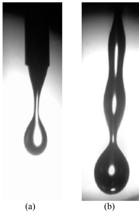
Figure 4: Drop formation in a co-flowing arrangement. The two modes of (a) dripping and (b) jetting are shown (from Cramer et al (2004)).
