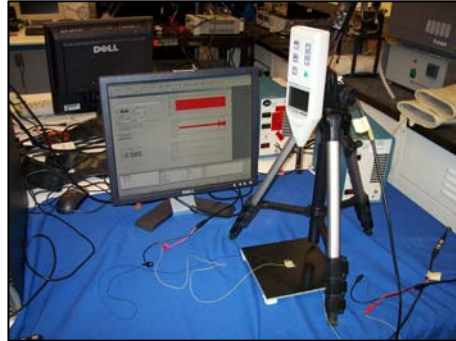
Figure 34: Acoustic vibration testing apparatus
