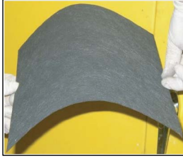
Figure 3: Carbon nanofiber paper
