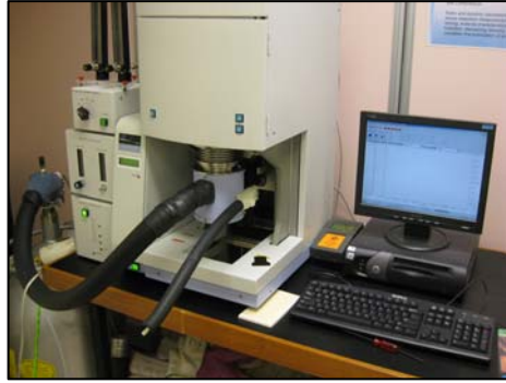
Figure 7: DMA testing apparatus
