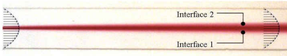
Figure 13 Progression of diffusion interfaces in the transverse direction to the flow; two interfaces are developed and move away from the centerline of the channel as one moves downstream
