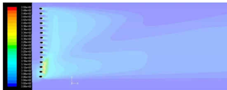
Figure 5.8: Temperature Contour of Case BR 1 Sr 0.1 at TS = 160, Spoke Location = 18.8°
