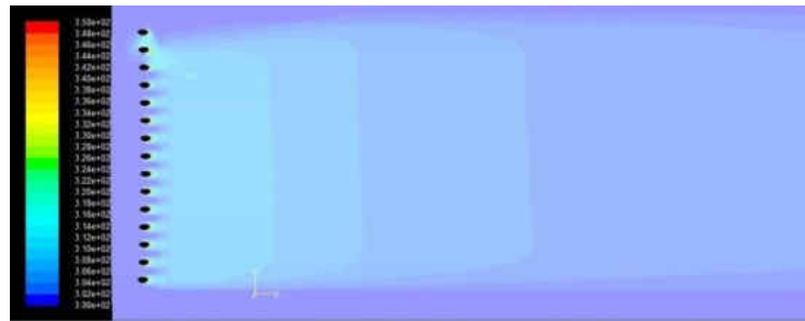
Figure 5.1: Temperature Contour of Case BR 1 Sr 0.1 at TS = 125 and Spoke Location = 13.2°
