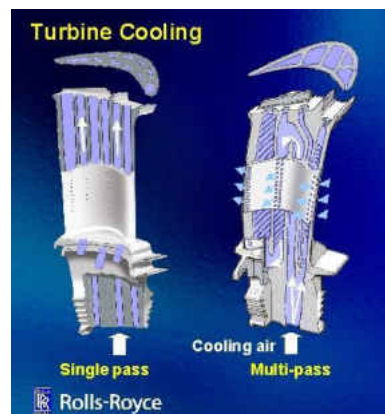
Figure 1.7: Rolls Royce Rotor Cooling Scheme
