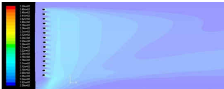
Figure 5.11: Temperature Contour of Case BR 1 Sr 0.1 at TS = 175, Spoke Location = 21.2°
