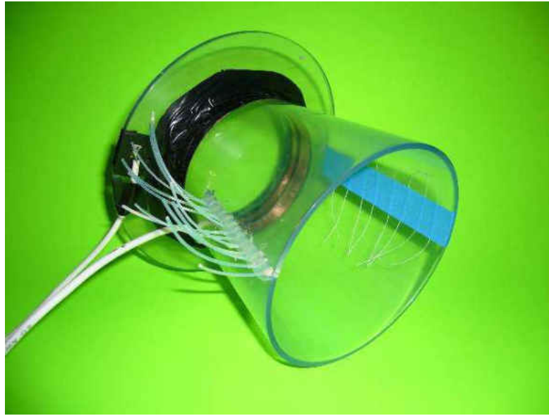
Figure 3.7: DBD plasma actuator arranged on diffuser model
