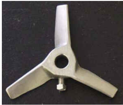
Figure 45: Lightning A-310 impeller
