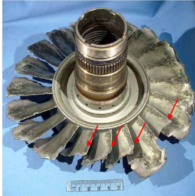
Figure 1.4: Failed first stage compressor row. From [9].
