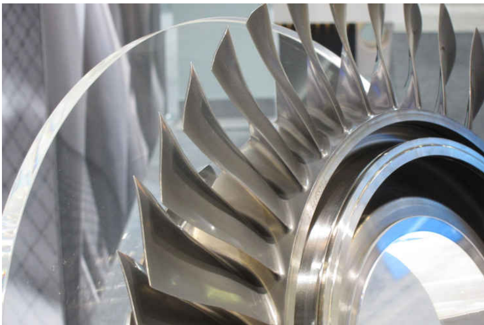
Figure 1.6: Monolithic construction. From [11].
