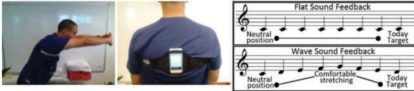
FIGURE 2. (Middle) Device attached to person's back for sonifying trunk movement during the forward reach exercise (Left). (Right) Examples of SESs for a forward reach exercise: The Flat sound is a repetition of the same tone played between the starting standing position and the maximum stretching position. The Wave sound is a combination of two tone scales (phrases), an ascending one ending at the easier stretching target and a descending one to the final more challenging target. The reaching of the easier target is marked by the highest tone (Singh et al., 2014).
