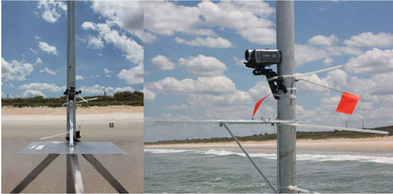
Figure 36: Lagoon rig with plexiglass water protection and camera installed, By Author, 2016
