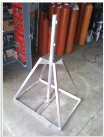
Figure 12: Welded frame of Turtle Cam Array at Superior Metals.
