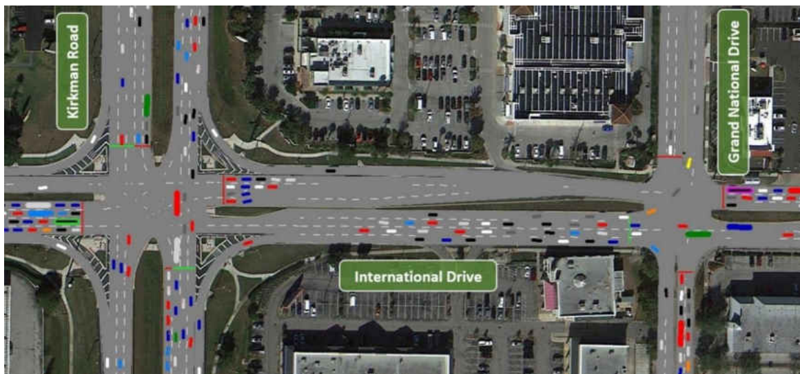
Figure 49: Kirkman (T2) and Grand National (T3) Intersections on I-Drive Corridor coded in VISSIM
