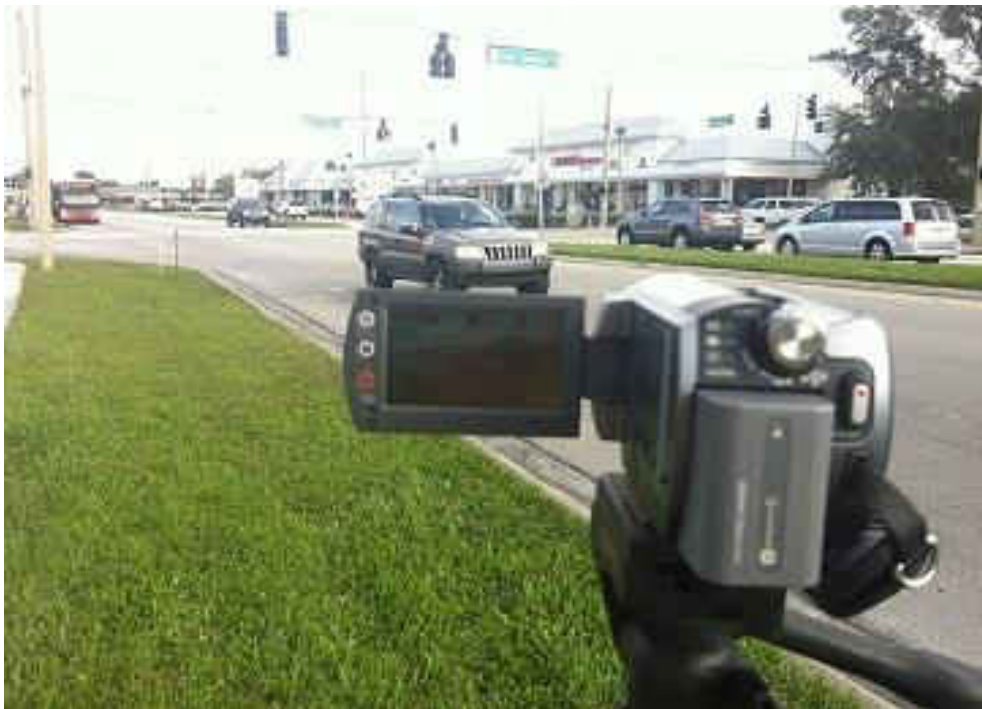
Figure 31: Videotaping Turning Movements (Camera Sample on T3 - Grand National with I-Drive Intersection)
