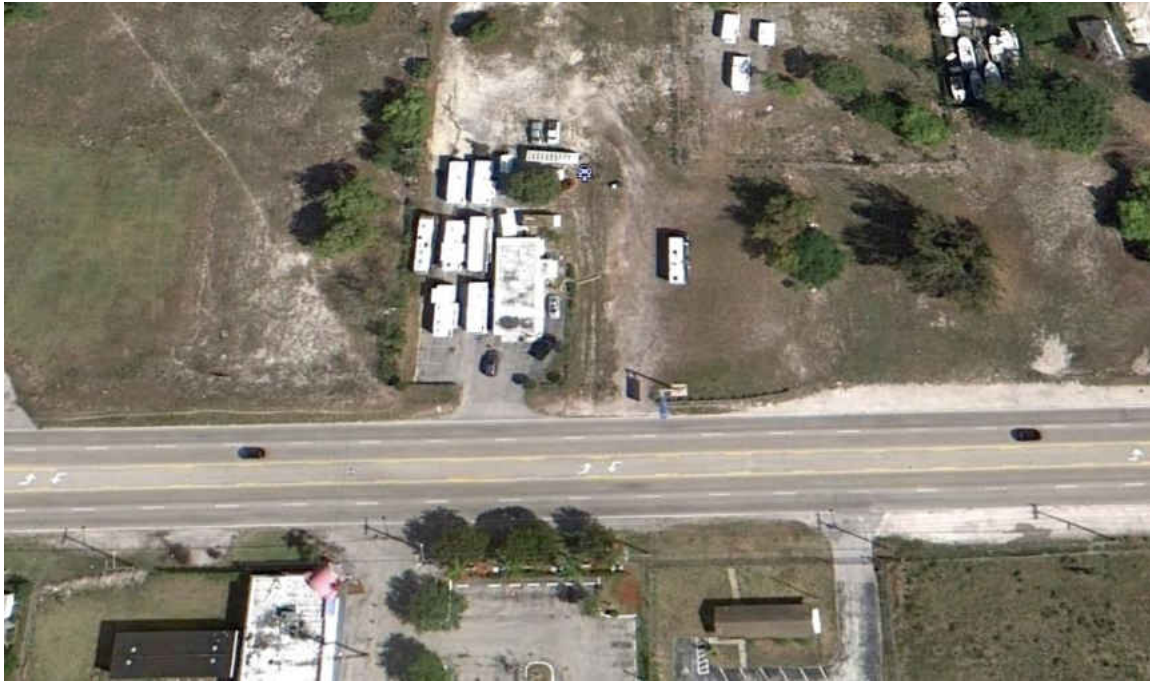
Figure 1-1: An Example of Two Way Left Turn Lane (TWLTL) Median (Source: Google Earth)
