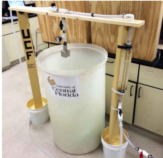
Figure 4.3 UCF Spray Aeration Bench Scale Unit
