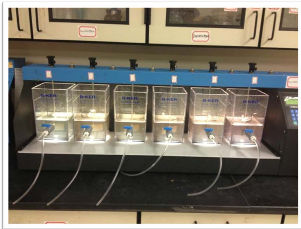
Figure 4-3: Potassium Permanganate Jar Test
