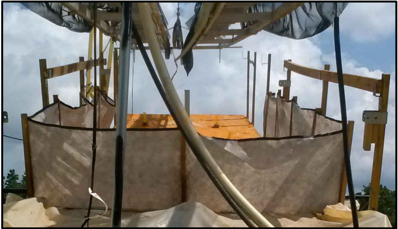
FIGURE 4 NONWOVEN (BSRF) SILT FENCE INSTALLED ON A TILTED TEST BED
