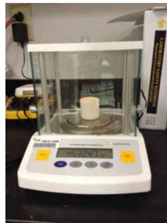
b. Cylindrical Alumina Crucible in the Measuring Scale
