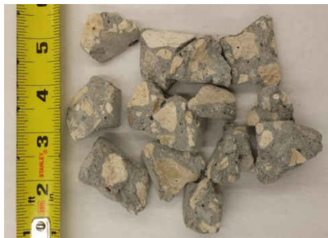
Figure 5.8: PCC specimen containing BA with particle size greater than 20 mm
