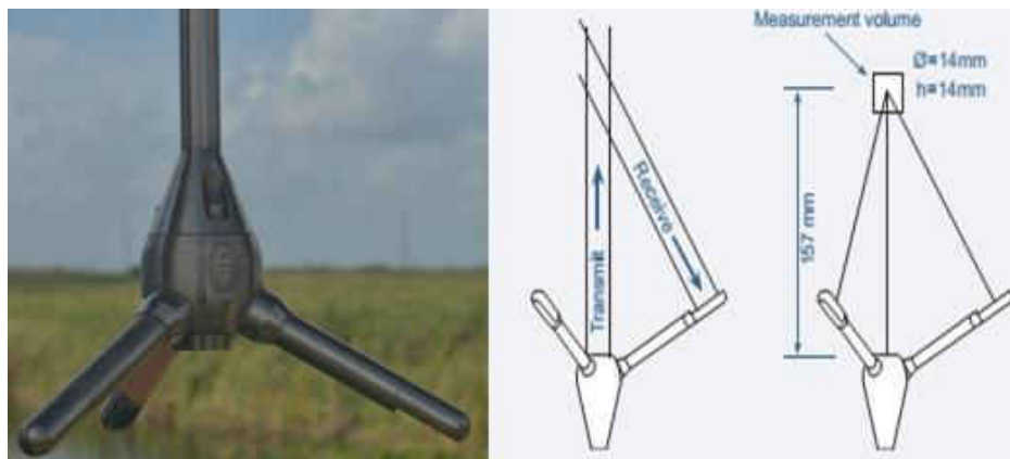
Figure 4.2: ADV sensor (left) and velocity measuring principle (right) (Nortek, 2005)
