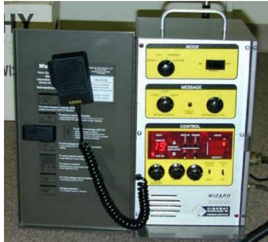
FIGURE 9 CB WIZARD ADVANCED WARNING UNIT (ULLMAN ET AL., 2002)
