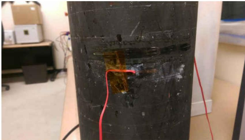
Figure 4:4: Installed Strain Gage on COPV
