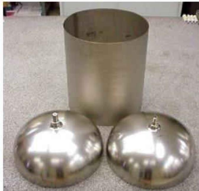
Figure 2:5: Components of the COPV Liner
