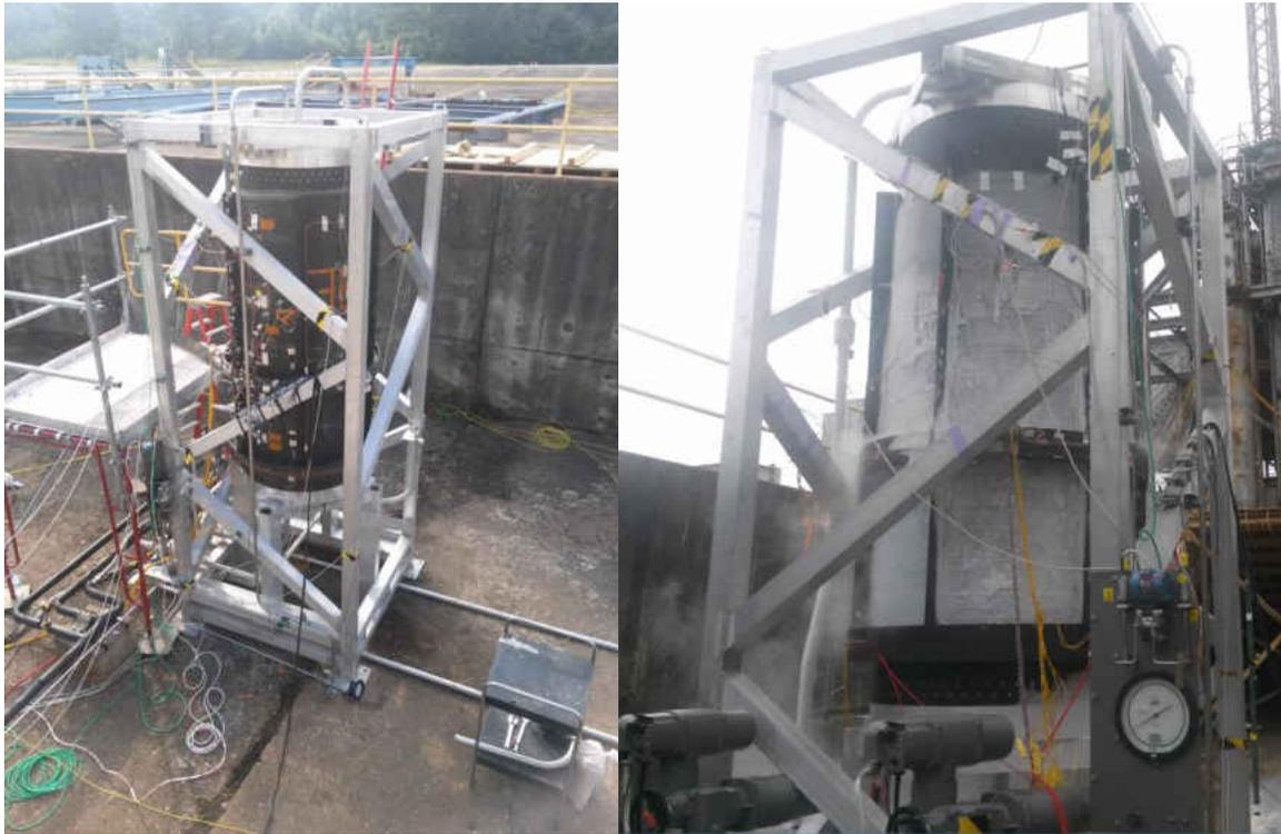
Figure 6:24: Instrumented AFRL Tank in Flame Trench (left) AFRL Tank Filled with LN2 During Testing (right)
