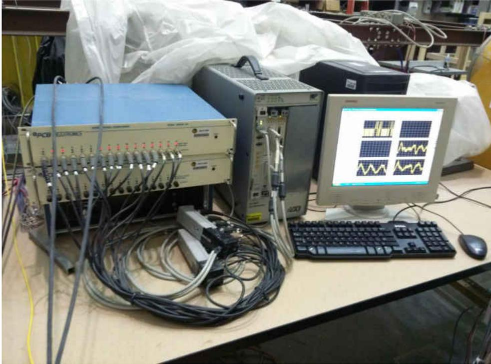
Figure 4:15: Dynamic Testing Health Monitoring System
