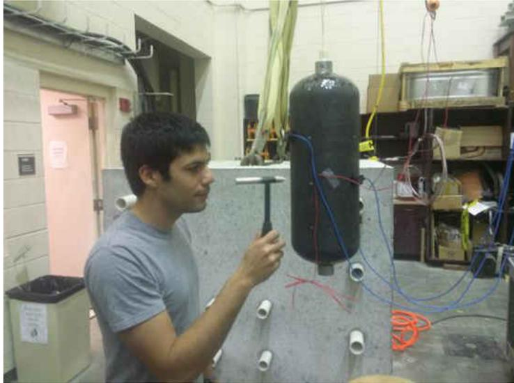
Figure 4:17: Exciting the COPV with the Impact Hammer
