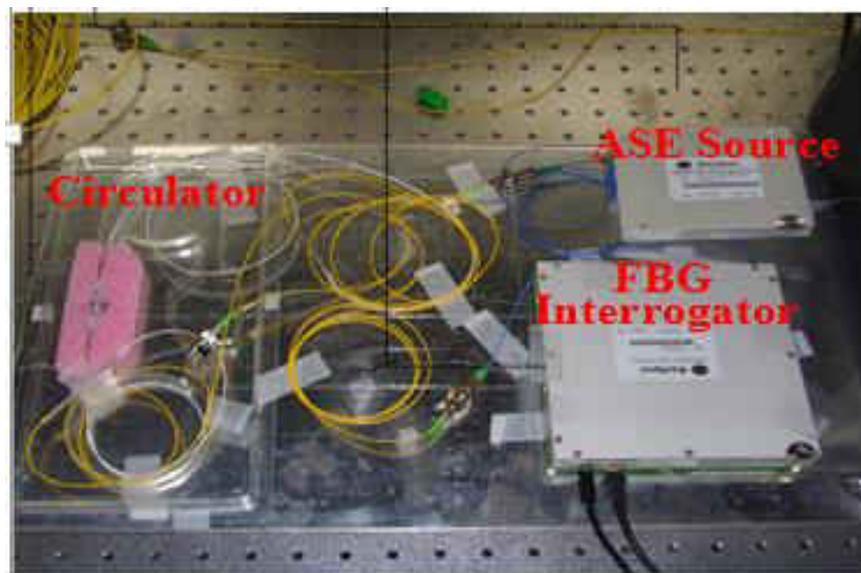
Figure 6:3: UCF In-House Developed FBG System
