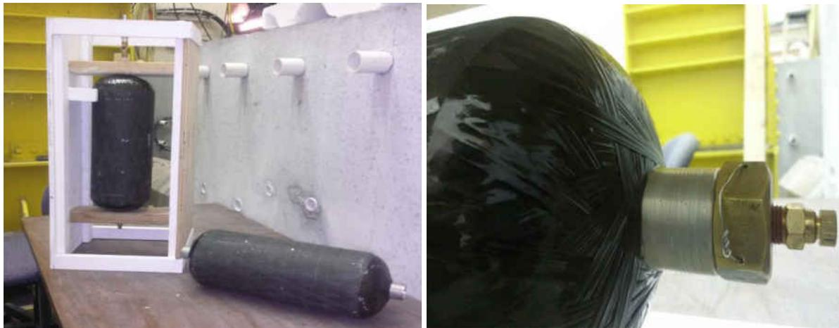
Figure 4:1: Two Test Specimens (left) COPV End Cap (right)
