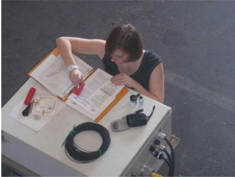
Figure 6:5: Mixing AE-10 Epoxy
