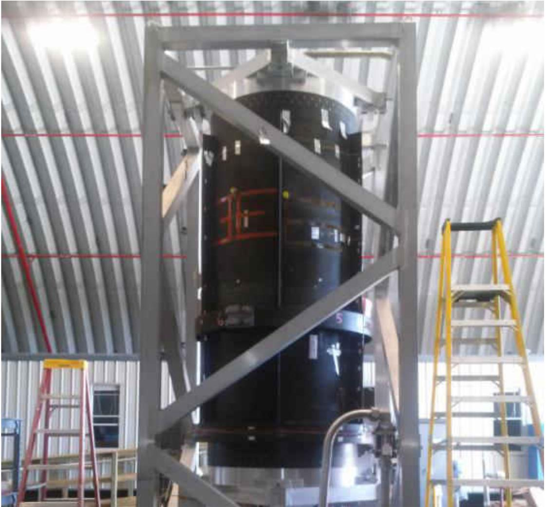
Figure 6:1: AFRL Tank in NASA's Clamshell Structure
