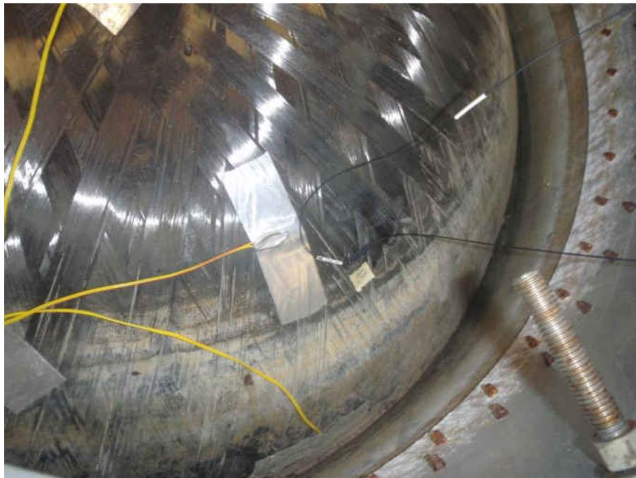
Figure 6:6: Installed FBG Sensor
