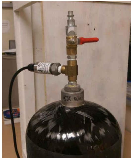
Figure 4:6: End Connection, Consisting of Pressure Transducer, Pressure Valve, and T-fitting
