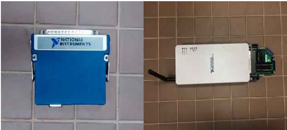
Figure 28. Pictures of the terminal block (left) and CompactDAQ Chassis connected to the DAQ (right)
