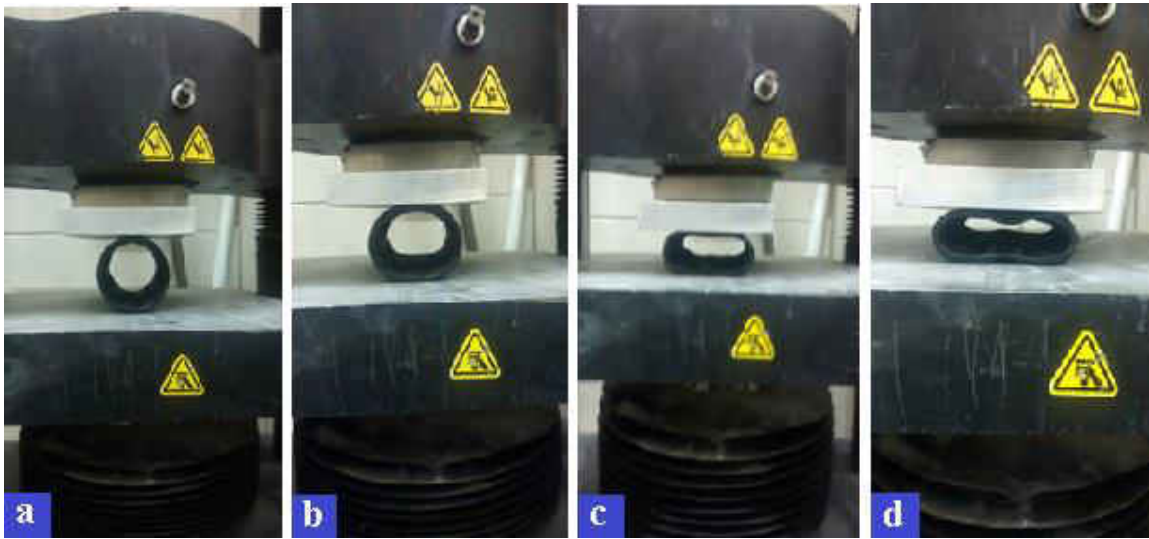
Figure 10. a. Single pipe before testing; b. Pipe is slightly deformed; c. Pipe is significantly deformed; d. Pipe is severely deformed
