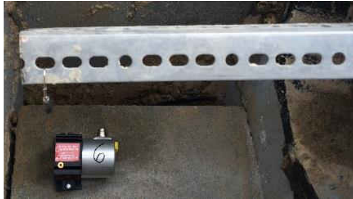
Figure 25. Connection between sensor and steel bar
