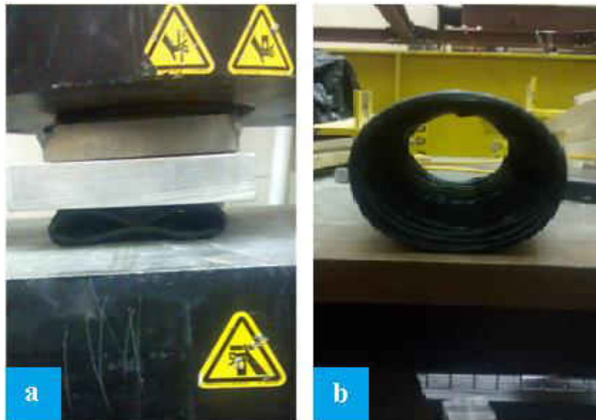
Figure 63. a. Severe deformation experience by the pipe; b. Pipe after a few minutes testing
