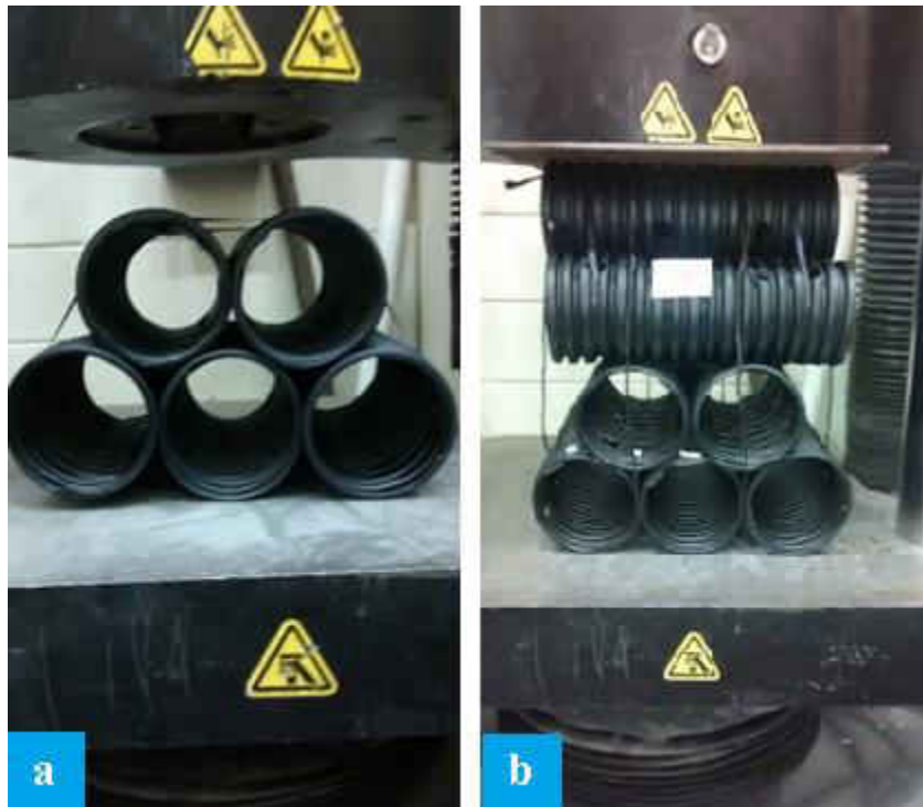
Figure 11.a. Single BPU before testing; b. Two-Level BPU before testing with top plate
