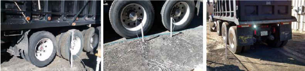
Figure 23.a. 2 rear axles and a dead axle; b. Two rear axles following the blue lines; c. Rear view of the truck driving away from the sensor's location
