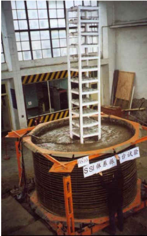
(a) A large-scale building model placed on soil foundation
