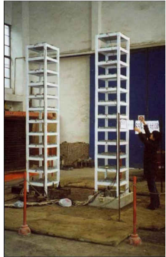
(b) Three identical reinforced cast-in-place building models tested in this study (two models are shown)
