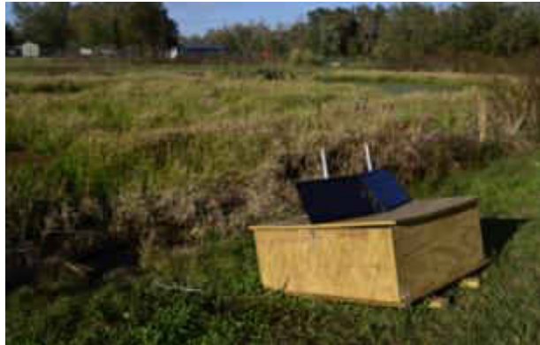
Figure 2-5 Exterior view of installation of SMBR on the pond bank at Zolfo Springs. The SMBR is powered by two 15W solar panels in parallel.
