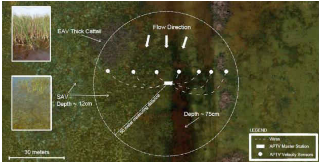
Figure 6-21 Theoretical field installation of APTV sensing network with seven velocity sensors positioned to capture horizontal velocity profile.
