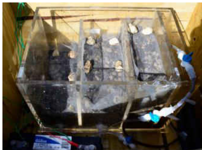
Figure 2-7 HMBR re-filled with 50% 5/8 th expanded clay and 50% tire chunk.
