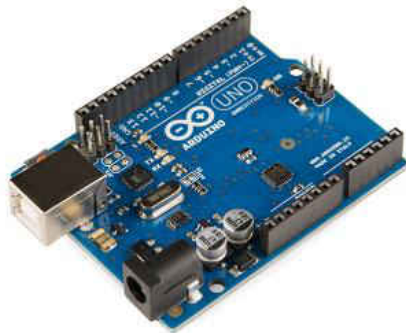
Figure 5-8 Arduino Uno microprocessor used for programming and control of the WASN collection units and peristaltic pumps.
