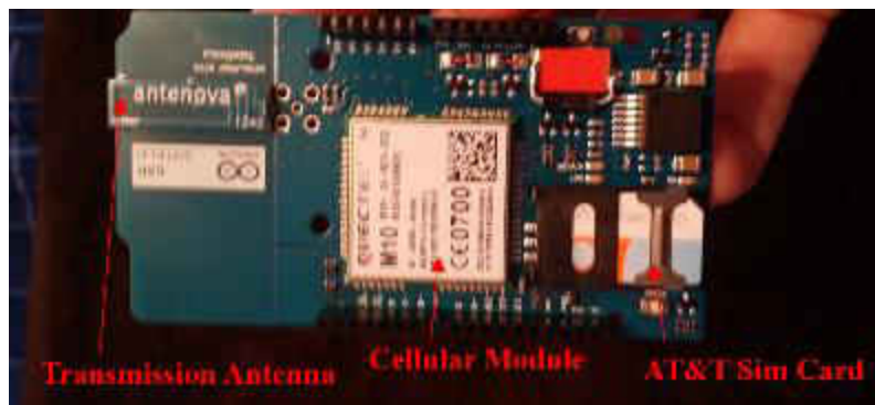
Figure 5-3 GSM module used for receiving text command and transmittal to XBee Pro.
