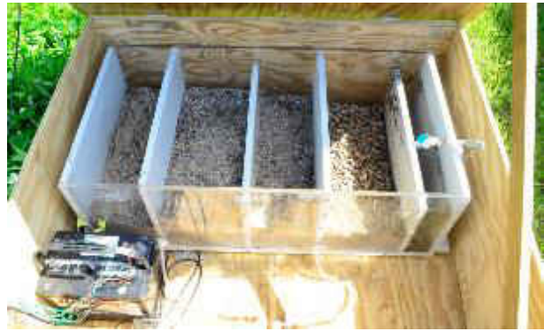
Figure 2-4 Installation of SMBR on the pond bank at Zolfo Springs with (a) without roughing media in the 1 st chamber and (b) with a 5/8ths expanded clay roughing media mix added to the 1 st chamber.
