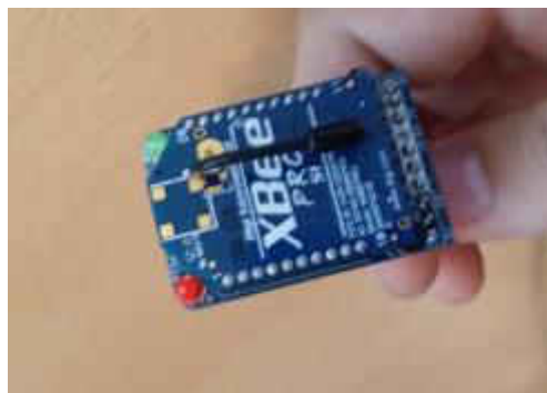
Figure 5-7 XBee radio transmitter/receiver used for communications between the GSM shield module and the sampling units. Each XBee has a maximum 1-mile transmittal radius.
