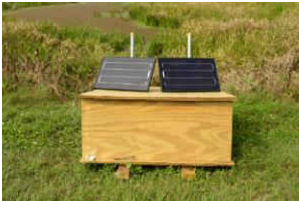
Figure 2-5 Exterior view of installation of SMBR on the pond bank at Zolfo Springs. The SMBR is powered by two 15W solar panels in parallel.
