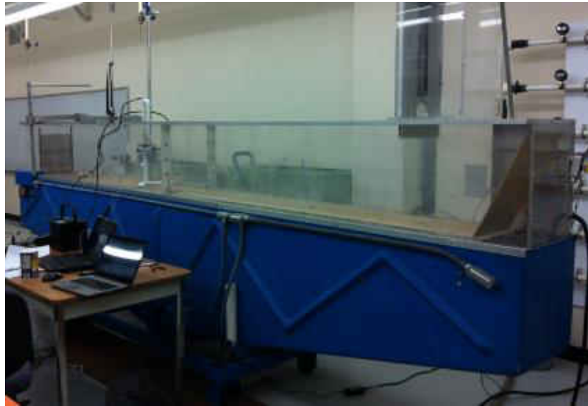
Figure 6-5 Picture of the Engineering Laboratory Design hydraulic flume used for the laboratory study. An APTV detector and Flow Tracker ADV are seen setup approximately three fourths from the beginning of the flume.
