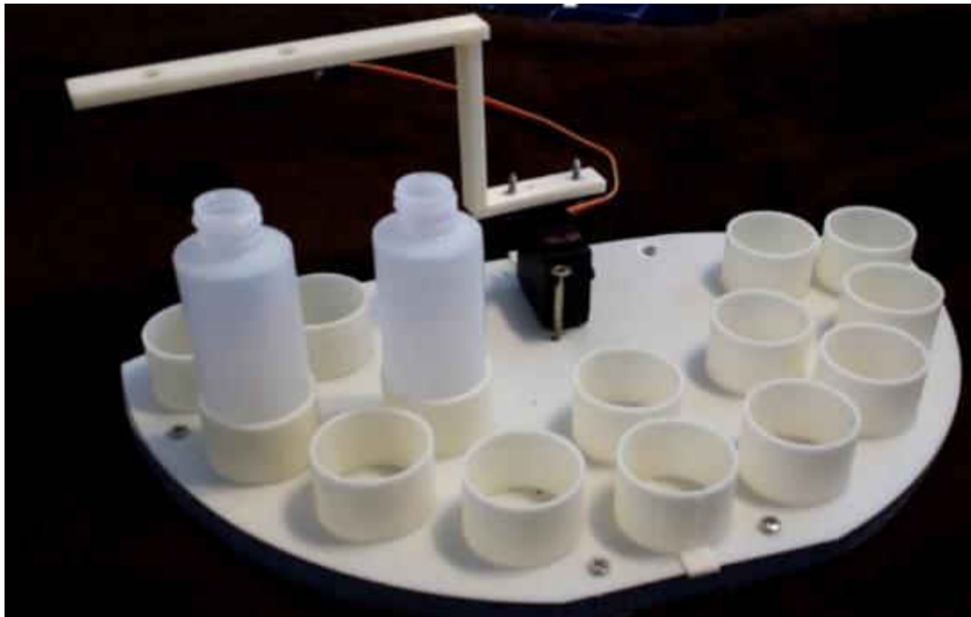
Figure 5-5 Photograph displaying the WASN sampling tray, servo motor and arm for holding influent tubes. The tray may hold up to 12 bottles (only two are pictured for clarity).
