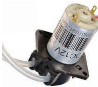
Figure 5-6 Adafruit high torque peristaltic pumps used for sample collection. Pumps operate on 12volt DC power and are directly powered by a battery.
