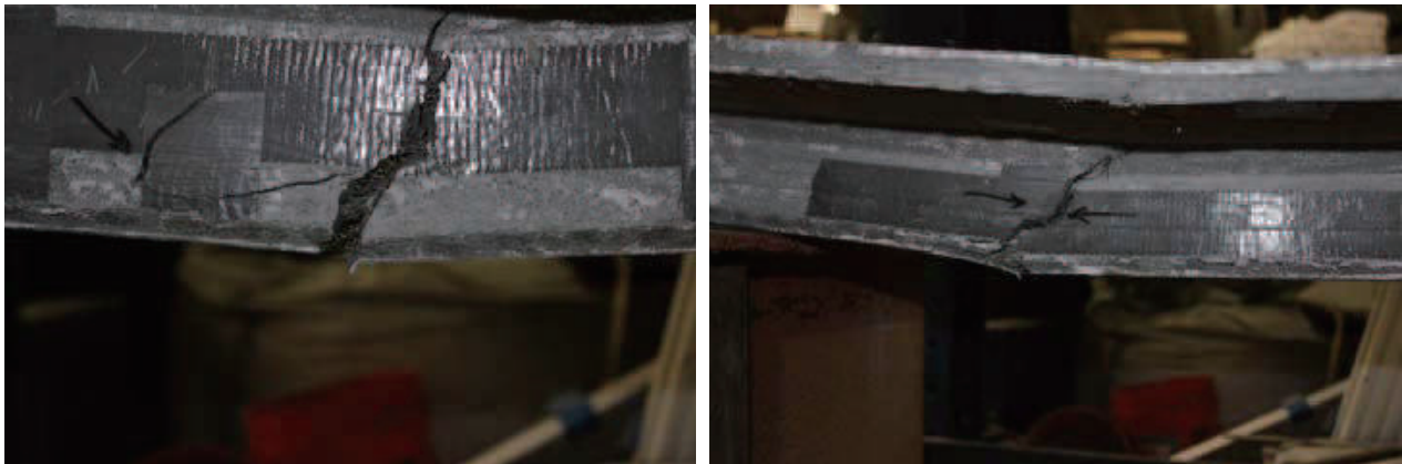
(a) Formation of flexural cracks in “UHPC-CFRP” specimen
