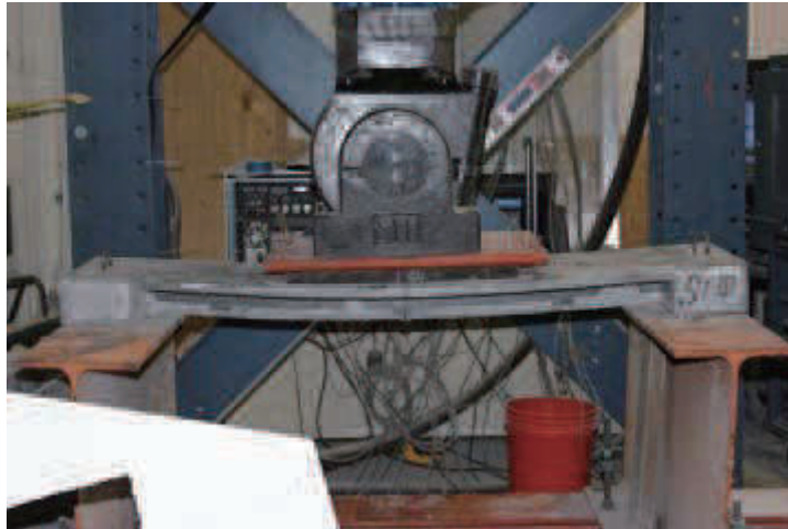
Figure 4.9: “UHPC-MMFX” specimen prior to failure
