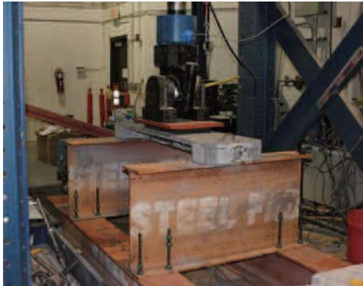
Figure 4.7: Test setup and instrumentation of “UHPC-MMFX” specimen
