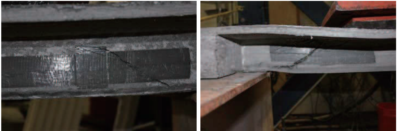
(a) Formation of shear cracks in “UHPC-MMFX” specimen (b) Shear cracks opening in “UHPC-MMFX” specimen
