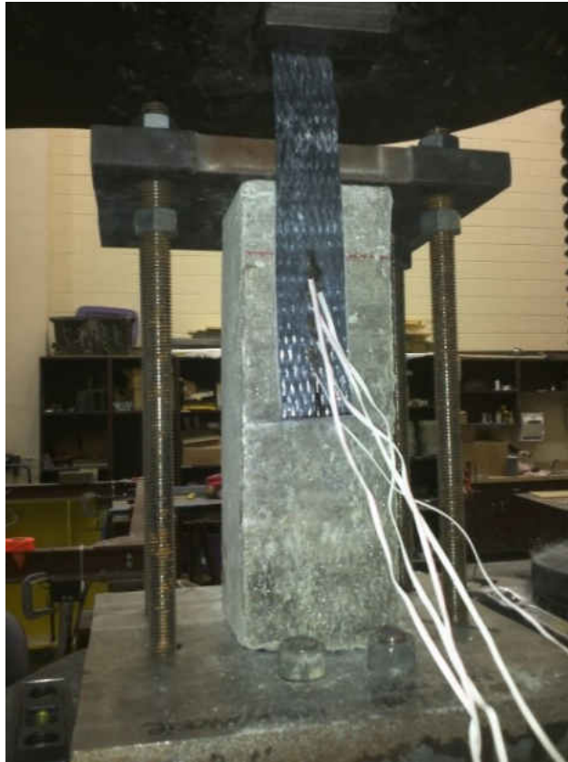
Figure 3.4: Lap Shear Test Setup Photo
