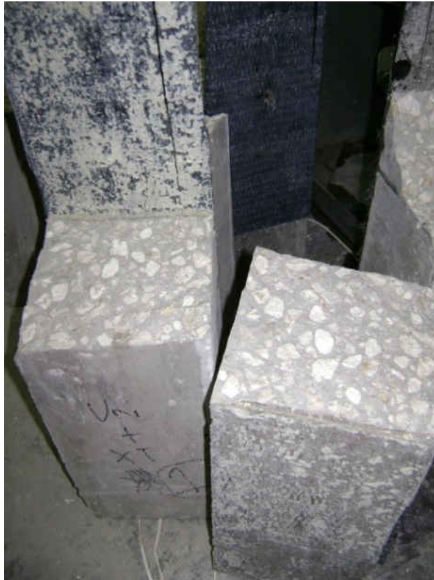
Figure 4.8: Polyurethane Uni + Ad1 De-bonding in Adhesive Layer
