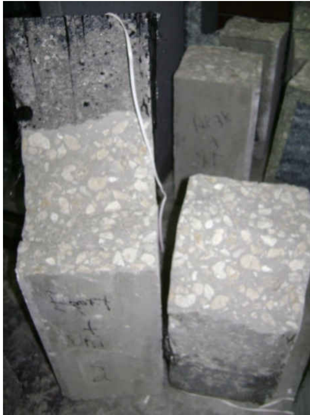
Figure 4.9: Epoxy Uni De-bonding in Substrate Layer plus Mixed mode Failure in Concrete
