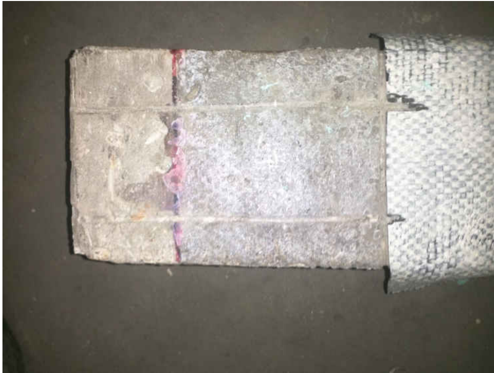
Figure 4.4: Photo of a Typical PU FRP Composite Lap Shear Failure
