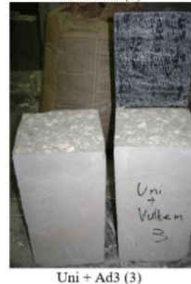
Figure A.3: Small Scale Flexural Beam: Uni Fibers + Ad3 (PU)
