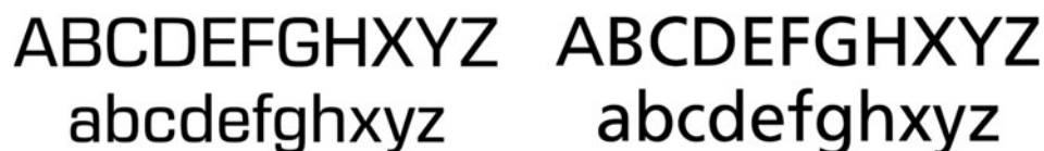
Figure 3. The fonts were constructed to have equivalent letter heights based on the capital letter ‘H’ in line with ISO 15008 standards for defining automotive font sizes. The square grotesque typeface (Eurostile) is on the left and humanist typeface (Frutiger) is on the right.
