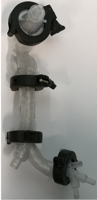
Figure 4. Three-dimensional cast printed using the SLA technique.
