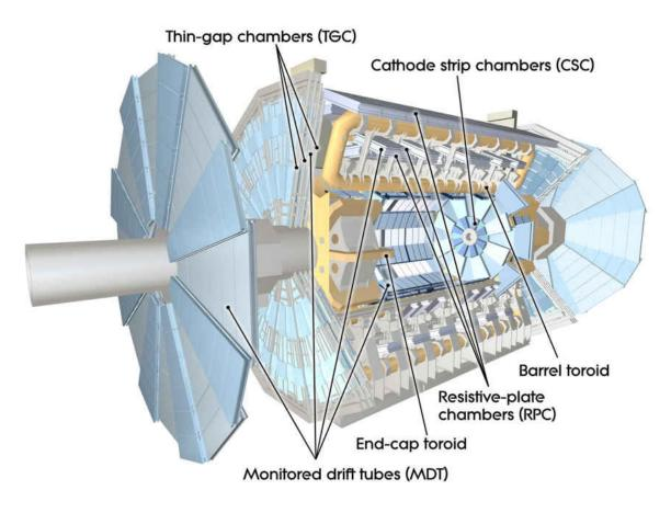
FIGURE 28. The ATLAS muon system [41]
