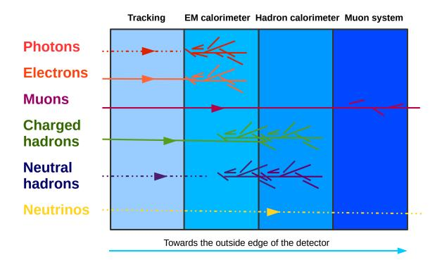
FIGURE 22. A cartoon of a cross-section of the ATLAS detector, and particle identification in each detector subsystem
