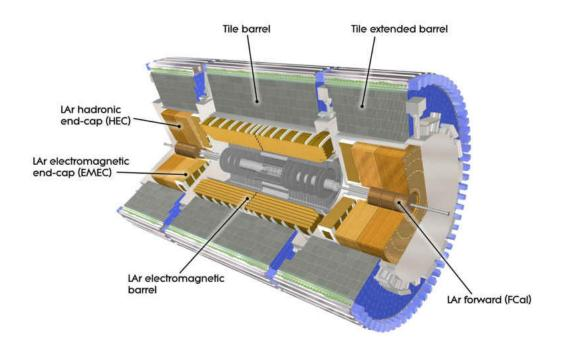
FIGURE 25. The ATLAS calorimeter [40]
