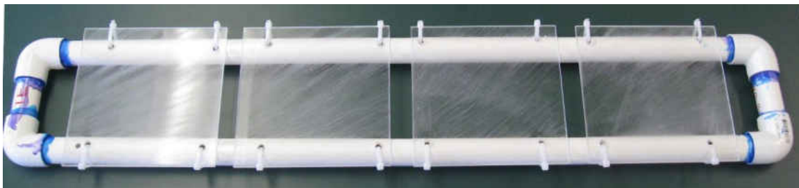
Fig. 38. Settlement plate deployment design. Individual plates are 15 x 15 cm.
