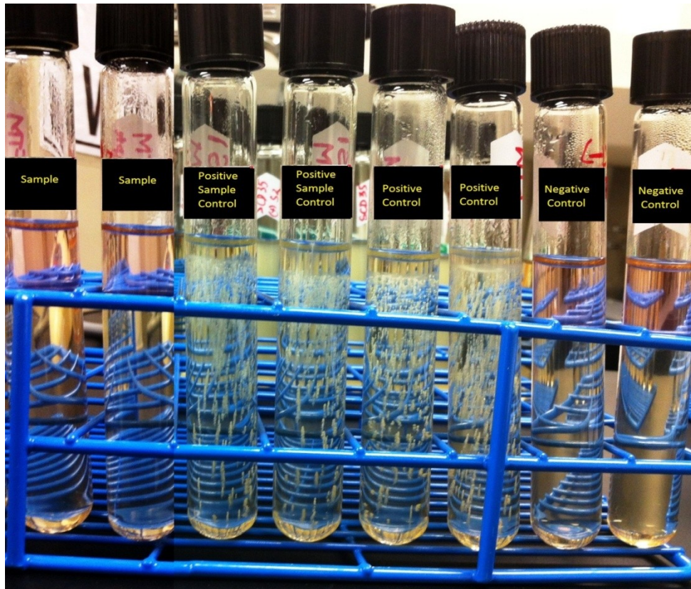
Figure 4-18: FTM tubes showing sample, positive sample control, positive control and negative control tubes, respectively after 24 hours of inoculation.
