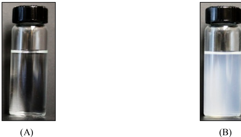
Figure 4-3: (A) A visually clear nanoemulsion and (B) a turbid and milky emulsion.
