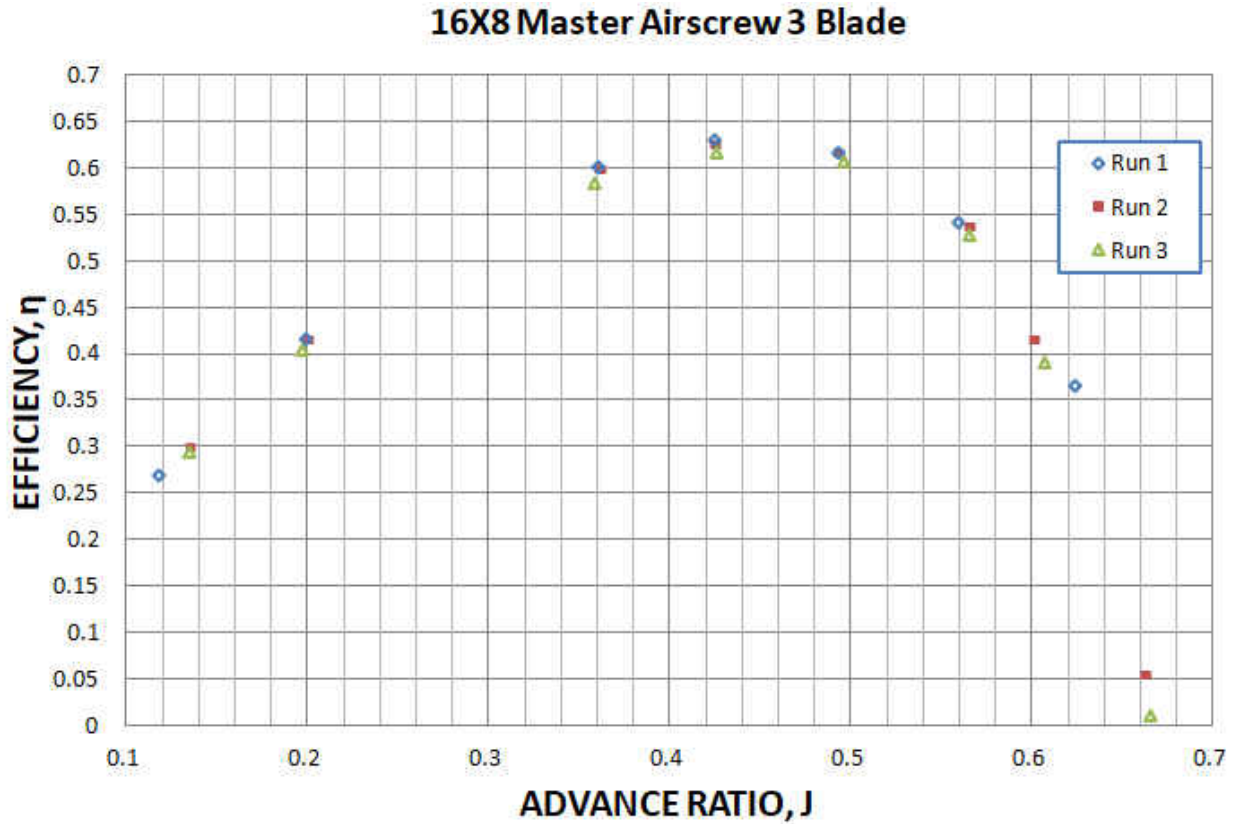
Figure 57: Efficiency Versus Advance Ratio
