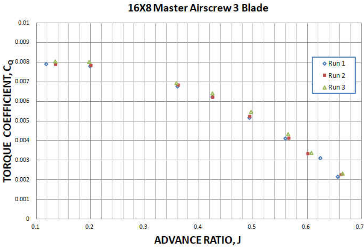
Figure 55: Torque Coefficient Versus Advance Ratio
